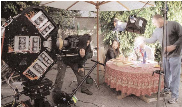
The Lockheed Martin Digital Cine Experimental Camera. The 4K camera system features RGB channels at 12 megapixels each and a 24p frame rate.
